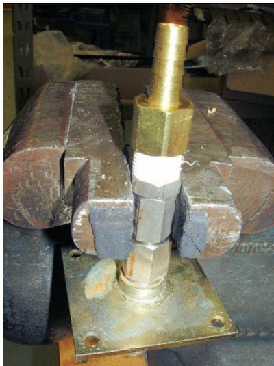
5. Wrap 5 turns of the Teflon tape around the 3/8" threads of stainless steel check valve fitting.
