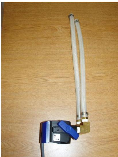
13. Cut the 2ft 6in length of braided silicon tubing in half into two equal 15" lengths
