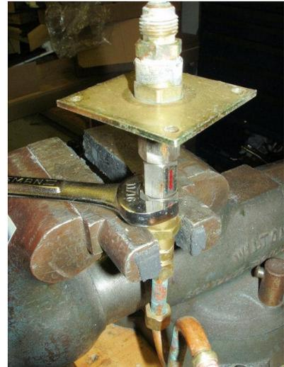
4. Remove the brass fitting that screws into the first stage of the Stainless Steel Check Valve as shown using the 11/16" wrench
