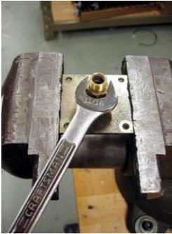
5. Using a 1 1/16" wrench, remove and discard the brass adaptor from the bulkhead plate
