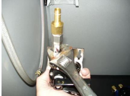
5) Remove the fittings from the original head using a wrench
