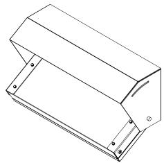
2. Mount the hood and display securely to the wall with the desired hardware and at the same time feed the harness through one of the larger knockouts previously punched out.
