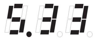
The display is only a single digit; therefore, to obtain the 3-digit error code the first digit is displayed WITH THE DECIMAL POINT (5.) and the second and third digits are displayed WITHOUT THE DECIMAL POINT (3) (3). The display will continue to flash the 3-digit error code; one digit at a time, until the failure is corrected or power is removed.
