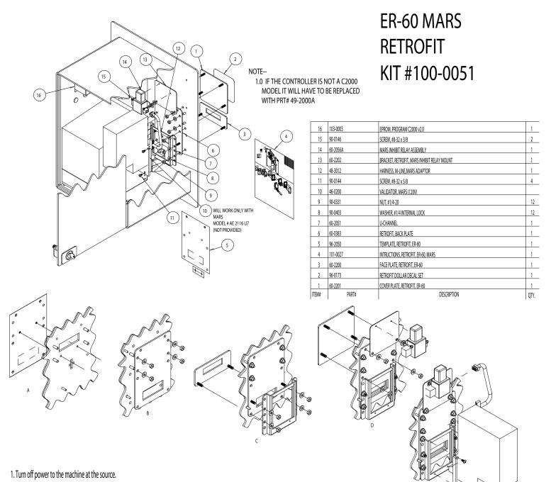
2. Remove validator, controller, stacker, stacker brackets, power box and harness from the machine. Be sure to then plug in the stacker bypass plug.
